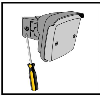
Tilt completely the sensor on one side to have access to fixing holes.
