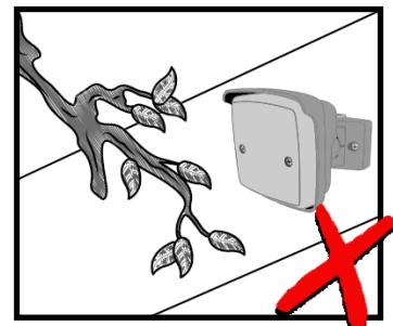
Objects such as fans, plants, etc must not protrude into the detection area.
