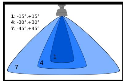
2. **Radar sensitivity:** Regulates the sensitivity and anti-interference filter. Starts from level 1 (maximum sensitivity + minimum anti-interference filter), to level 7 (minimum sensitivity + maximum anti-interference filter);
