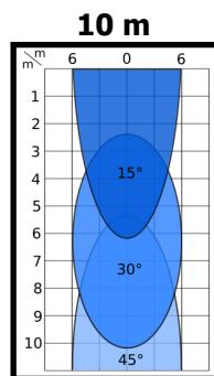
All detection field dimensions were measured in optimal conditions with default field size value
